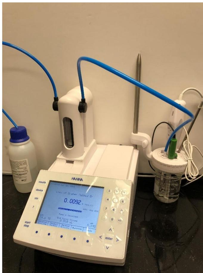
Figure 9: Setup for titrations conducted with the potentiometric titrator, Hanna Instruments HI931.
